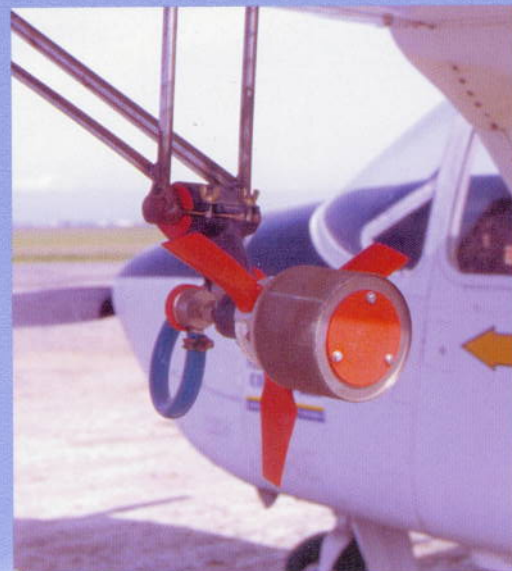
Micronair system setup for mosquito control
